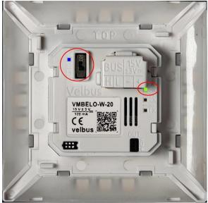
Tapping the button surfaces on the front of the panel will light up the TX LED (sending CAN bus data). Using another device in your Velbus installation should light up the RX LED (receiving CAN bus data). Use these LEDs to troubleshoot if your Velbus control panel is properly connected into the Velbus network.
