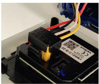
When your Velbus installation is powered, you should see a green LED next to the **PS** label. The blue LED next to the TERM label indicates that the terminator is closed (switch set into the upper position). This should be the case if your Velbus control module is at the end of a EIB cable. If the Velbus control module is in series with another device, the terminator should be opened (switch set into the lower position – blue LED will not be activated).
